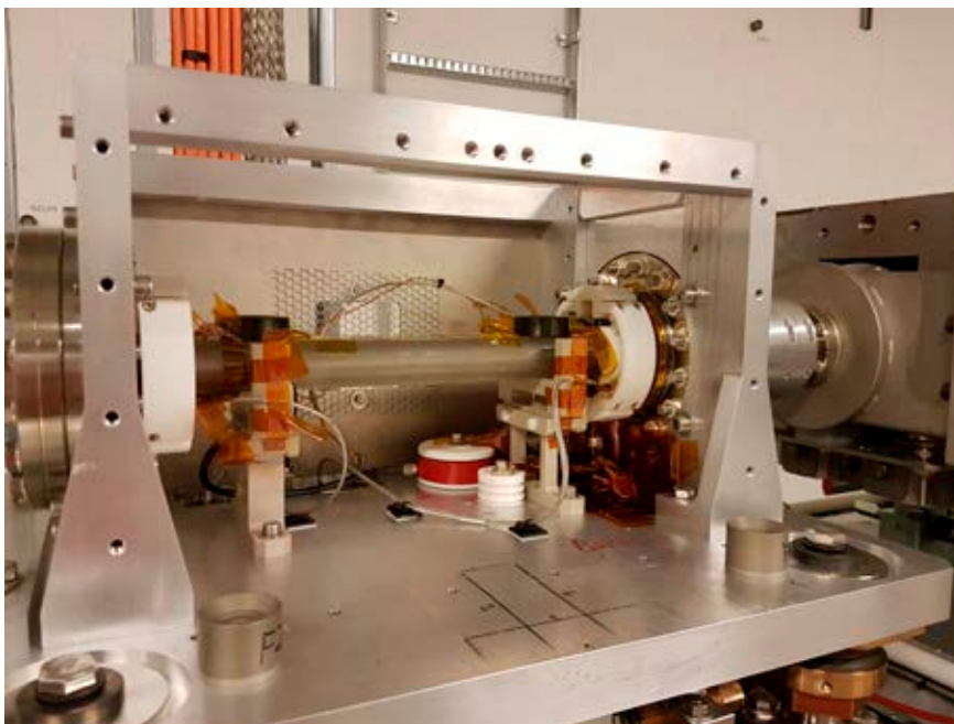
Figure 4: The Multipole Injection kicker installed in the 3 GeV ring. An identical component is planned for the 1.5 GeV ring.
