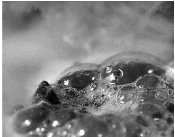
Hydrogen gas is generated as one of the products between aluminium and an acid.
