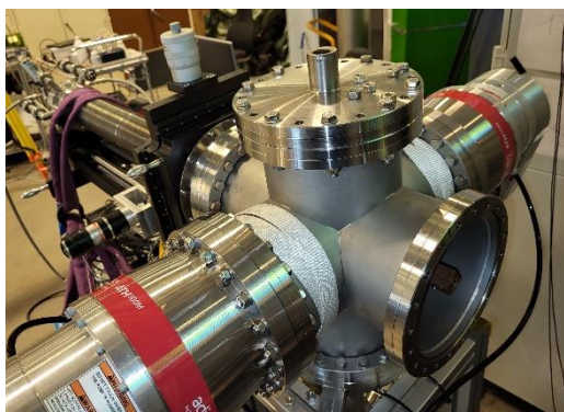
Figure 2.15: Molecular/cluster beam setup with the 50-micron nozzle for gases (not vapours) mounted. The setup is built on a commercial 6-way CF160 cross with two ATH-500 maglev turbo-pumps backed by a corrosive-gas and moisture resistant dry forevacuum pump. The nozzle is mounted at the tip of the rod held by an XYZ VG Omniax 400-mm Z-drive manipulator. The nozzle can be replaced by a heated vessel for producing beams of molecules and clusters out of liquids.
